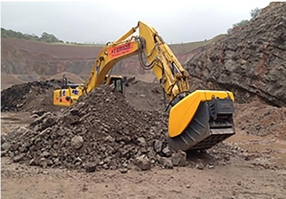
The reduction rate of the material to be crushed versus the bucket opening length **has to be** maximum 1:6. For example, if the jaw opening setting is adjusted 0.78 in., the maximum length of the material to be crushed is 4.75 in.
