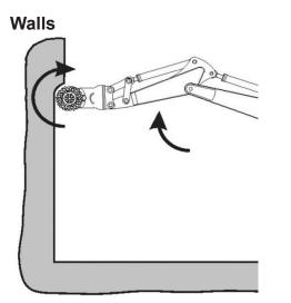
When operating on vertical surfaces, the Cyclone must be turned 180 degrees to reduce vibration and counter-forces during cutting.
