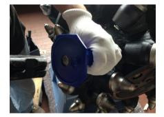
Break up the C-retaining ring using a hammer. Use the installation tool for the securing ring.
