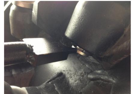
Loosen any stuck picks by driving the wedge into the gap between the pick and the holder.
