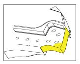
Yellow area - when necessary, build up the front lower edge of the tang and the front vertical surface of the upper. After welding, surfaces should be squared with a grinder and finished with a file and machinist's straight edge.
