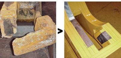
Component restoration, parts replacement and complete attachment rebuilding
