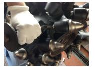
Knock the pick out of the holder using a hammer and a reaming tool.
