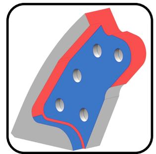
When necessary, build up the front lower edge of the tang (areas **highlighted in yellow**), following the procedures in the [GXT Safety and Operator's Manual](#). After welding, surfaces should be squared with a grinder and finished with a file and a machinist's straight edge.
