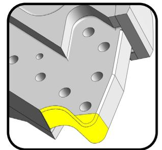
Piercing blade bolts must not make hard contact with the bolt holes in the upper tang. In rare cases, it has been noted that improper alignment of piercing blade bolt holes and the bolt holes in the tang can cause the piercing blades to break through the bolt holes.
