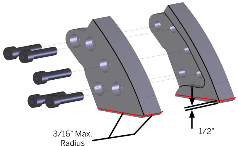
6. Typical use requires blade replacement at approximately 200 hours; heavy piercing requires replacement at approximately 40 hours. These are general guidelines only. Replace blades based on wear not hours of operation.
