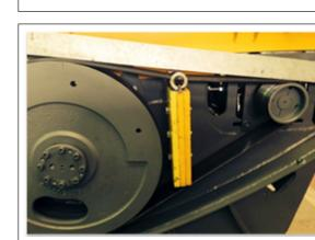
Inspect the belt tension. Optimum displacement is 0.40 in. If less, loosen belt tension. If more, tighten belt tension.
