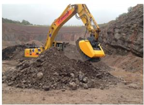
The reduction rate of the material to be crushed versus the bucket opening length **has to be** maximum 1:6. For example, if the jaw opening setting is adjusted 0.78 in., the maximum length of the material to be crushed is 4.75 in.
