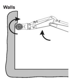
When operating on vertical surfaces, the Cyclone must be turned 180 degrees to reduce vibration and counter-forces during cutting.
