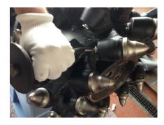
Knock the pick out of the holder using a hammer and a reaming tool.
