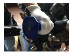
Break up the C-retaining ring using a hammer. Use the installation tool for the securing ring.
