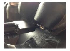
Loosen any stuck picks by driving the wedge into the gap between the pick and the holder.
