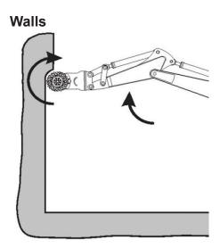
When operating on vertical surfaces, the Cyclone must be turned 180 degrees to reduce vibration and counter-forces during cutting.
