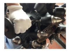
Knock the pick out of the holder using a hammer and a reaming tool.
