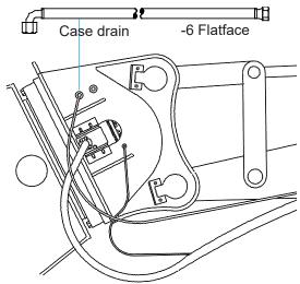
Use the correct fittings. Secure the case-drain line to the excavator stick.
