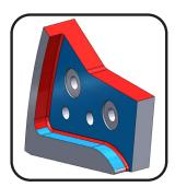
When necessary, build up the front lower edge of the tang (areas highlighted in yellow), following the procedures given in this manual. After welding, surfaces should be squared with a grinder and finished with a file and a machinist's straight edge.
