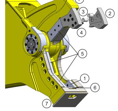
7. Jaw hard-surfacing - build-up and hard-surface as needed.
