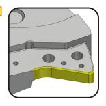
It is critical that the tip blade pocket and tang surfaces are straight and true, without dings, deformations, high or low spots, or areas that are worn away.
