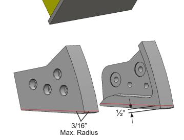
7. Width of blades, top to bottom, may taper 0.060" (2 mm) total. Bottom edges may be worn to a maximum radius of 3/16".
