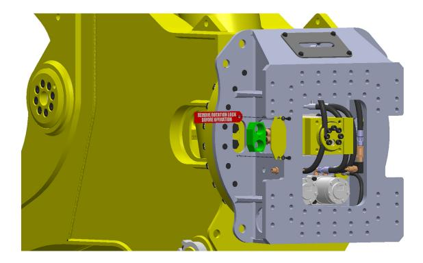
Rotation (transport) locks are installed at the factory to allow the bracket to be shipped with the mounting pins facing upward. This is beneficial to the end user when removing the attachment from the truck and mounting it to the excavator.
