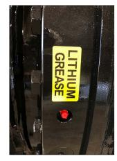
Genesis GLG-2® anti-wear, extreme-pressure lithium grease, PN 6302601, is recommended for all temperature conditions.
