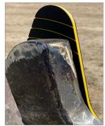
Properly maintaining demolition attachment teeth maximizes performance and optimizes the life of replacement parts. As teeth become worn, they need to be rotated, built-up or replaced.
