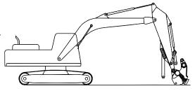
Position the excavator behind the attachment and carefully line up the stick connection of the excavator and attachment. Install pin.
