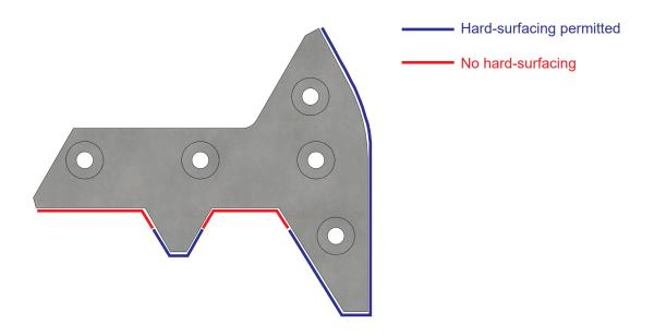
Hard-surfacing in the red areas can lead to premature tooth failure. Always build-up/hard-surface with the grain of the tooth. Do not weld across the tooth. Hard-surface material should have less than 10% chrome content and be applied on top of a 7018 root pass.
