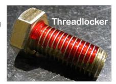
For thru holes or nuts, apply threadlocker to bolt threads.
