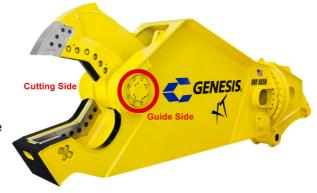
End cap bolt failure can also result from processing high-strength cable. The cable will not cut completely once the blades are dull and will wedge between the upper and lower main cutting blades. This puts extreme force between the blades and pushes the main shaft sideways into the end cap, popping off the bolt heads.
