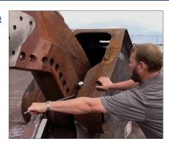
The main bearing will wear more on the cutting side, causing the main shaft to start twisting toward the bearing on the guide side. The end of the main shaft will then contact the thrust washer under the cap at an angle instead of flat against it. This results in point-loading that will cause the end cap bolt heads to fail in the 6 to 9 o'clock positions on the end cap.
