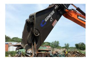
Insufficient gaps between the piercing blades and guide blades subject the blades and jaw parent material to thermal expansion from cutting friction. The tighter the blades run, the hotter they get and the more they expand.
