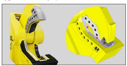
Piercing blades and guide blades are the most susceptible to this and will show blue streaking on their faces. In some cases, they will get so hot that surface cracks and spidering occur. The heat and blade expansion also spread the lower jaw and increase the gaps between the primary and secondary blades, causing thin material to jam between them.
