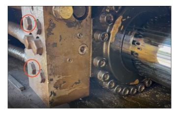
in both directions to see if oil is coming up through the threaded cylinder bolt hole. If oil is coming through, the cylinder head-to-barrel seal has failed. If not, reinstall the bolt to factory torque spec.
