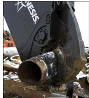
Check blade bolt torque, gaps and wear every day while at ambient temperature before startup. Re-torque loose and replace broken bolts.
