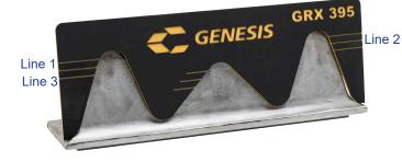
To help customers determine and monitor how far processor teeth have worn from their original shape, Genesis has created tooth build-up templates.
