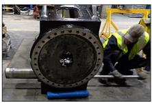
Push the cylinder to the back of the shear. Lift the cylinder, barrel end clevis first.
