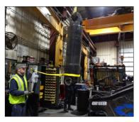
When you reinstall the cylinder following maintenance, be sure to use new O-rings coated with clean grease. Torque and Loctite 262 application specifications can be found in the **GXT Safety and Operator's Manual** and the **parts manual** for your shear model.
