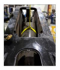
Retract the barrel slowly to avoid damaging the auto guide assembly with the cylinder clevis.
