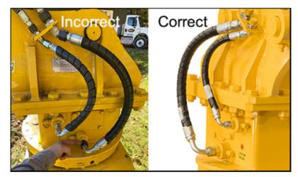
Hoses that are twisted when the fittings are tightened may also come loose as they will want to twist counterclockwise when they pulse under pressure. This is something we see quite regularly, especially with rotation jump lines from the carrier to the attachment. Tightening a twisted hose will cause the hose connection, bulkhead fittings, and flow control connections to come loose. A hose that is twisted may also prematurely fail in the area that is twisted or at the fitting.
