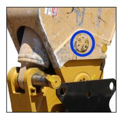
If any hose or component, such as the swivel or lock-pin cylinder, has been removed, serviced or replaced but not properly reinstalled, the lock-pin will extend but not retract.
