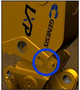
If this occurs, remove the hoses and fittings connected to the lock-pin cylinder and the two large socket head screws holding the cylinder into the center tube. Slide the cylinder out of the
