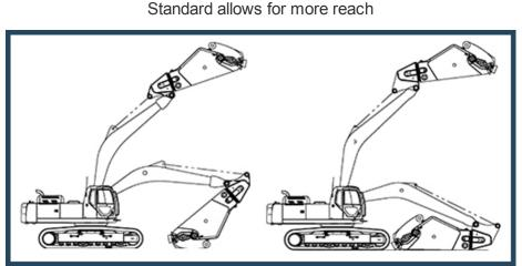
Transport bracket designs allow for ease of mobility or maintenance without having to unpin the stick cylinder.
