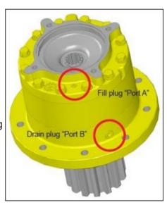
Add lubricant through the fill plug to 1-1/2" from the top of the fill plug (Port A). Do not overfill. The gearbox oil level should be 1-1/4" to 1-1/2" below the fill plug with the gearbox positioned vertically.
