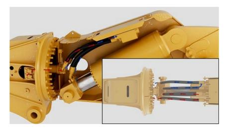
Excavator spools, which control oil flow, open and close by sliding back and forth inside the control valve spool bore. Control valve spool position is a function of the excavator, controlled by the operator, and not a function of the shear. A shear will not perform properly if this operation is compromised.
