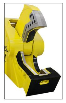
Genesis Shear Jaw Armor® is a proprietary plate system designed to be a sacrificial wear surface that takes the brunt of the shearing forces and abrasion in high wear areas of the upper and lower jaws.
