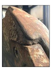
Retro-fitting Jaw Armor onto well-used shears is also extremely difficult due to the worn jaw surfaces and need for precise fitment. In many cases it can be done, but time and care must be taken to ensure the Armor fits as intended.
