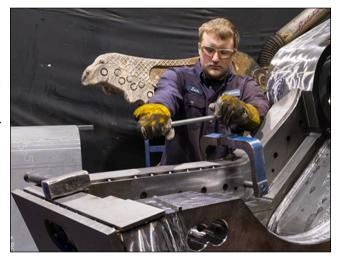
Hard-surfacing over Jaw Armor components is not recommended. The welding may cause buckling of the plates as they cool, creating an unwanted void between the Armor and jaw surfaces, and allowing for movement that will likely lead to weld failures caused by compression during cutting.
