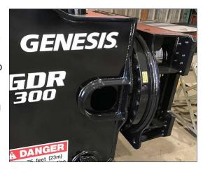
Rotating components must be greased daily. Grease fittings are located on the outside of the slewing ring and on the inside of the rotating head assembly. Grease locations are marked with decals.
