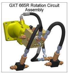
A cross-over relief valve may get stuck open between the plunger and nose if tiny pieces of debris get caught while the valve is open. This will cause the rotation motor to suddenly stop working.
