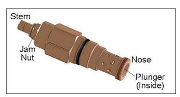
Turn the stem back to its original position and snug the jam nut. Install the valve back into the motion control manifold and torque to 150 ft lbs.
